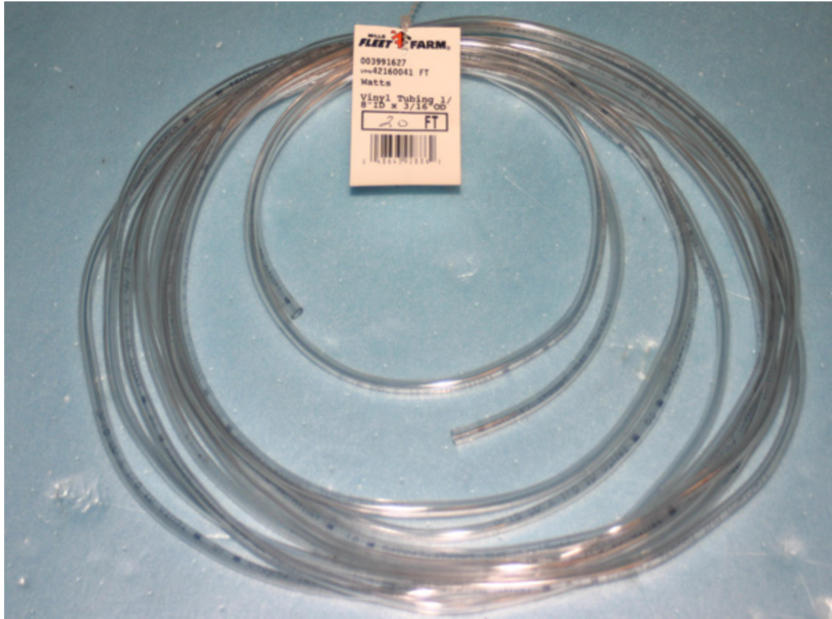
1/8" ID x 3/16" OD Tubing Fits the Syringe Tight
