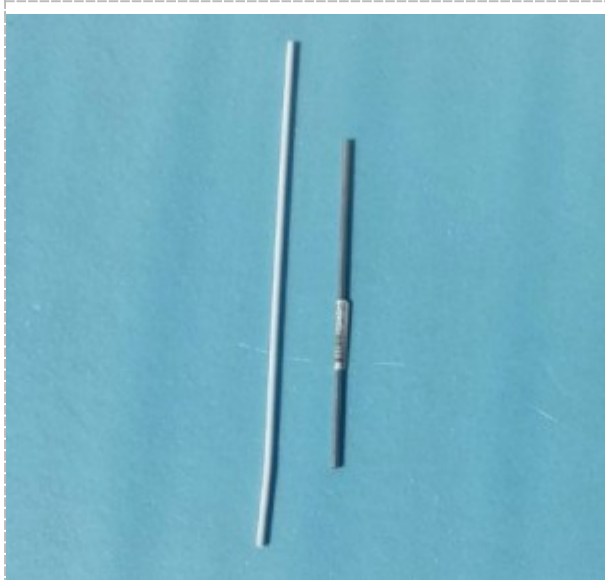
1/8" ID x 3/16" OD Tubing Fits the Syringe Tight
