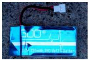
done several tests on both of mine and find consistent and disappointing results. Although they performed satisfactorily, all dimensions and test results indicate that these batteries must have an actual rating of about 550 mah, which is way shy of their labeled and advertised 720 mah rating. I am in ongoing dialog with the dealer to cease sale of this battery. Of course he passed the buck to his supplier. Buyer beware!
