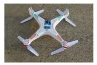
The "fully-dressed" configuration sports the quad complete with its landing skids, blade guards, battery door and camera. The camera was not activated in these tests, however,
